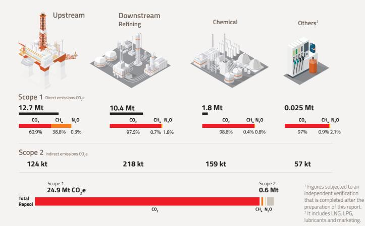
Scope 1 (Direct emissions). Scope 2 (Indirect emissions associated with purchasing electricity and steam).
